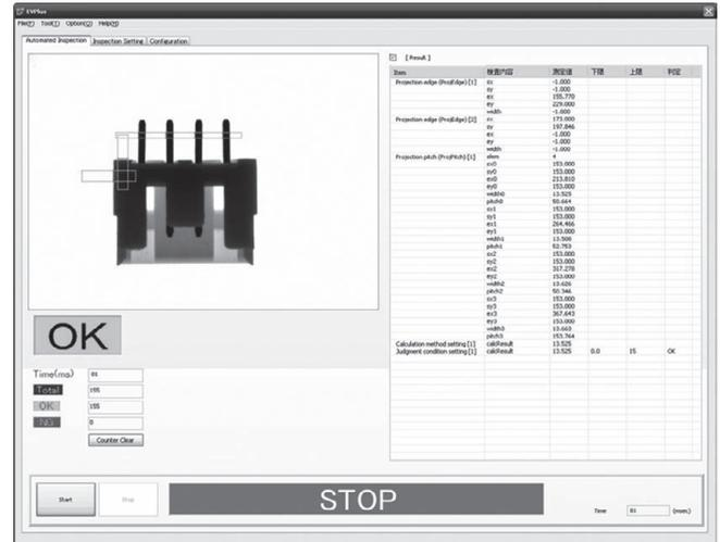
Fig. 10: Screen layout of the EV-Plus software
