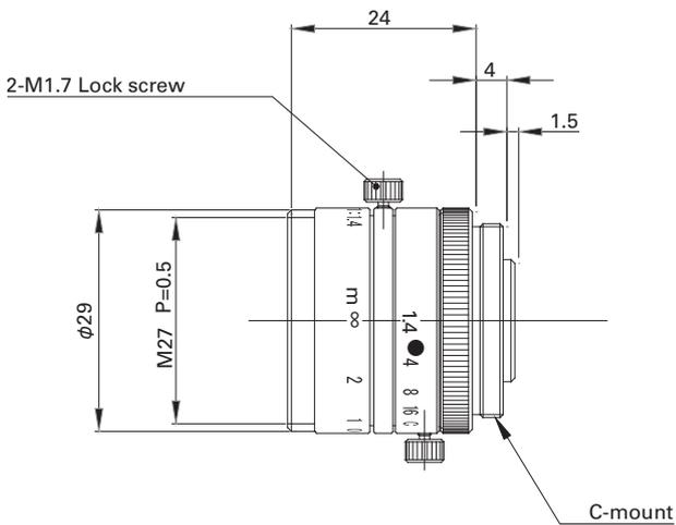
Fig. 4: External diagram of the lens
