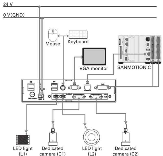
Fig. 9: Example of system connection for the “VS-EV”
