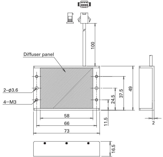
Fig. 5: External diagram of the flat-type LED light
